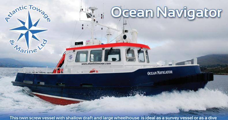
This twin screw vessel with shallow draft and large wheelhouse is ideal as a survey vessel or as a dive support vessel, also with her new winch tow hook crane & A-frame it makes her a very versatile workboat/inshore tug and is perfect for a variety marine operations.
