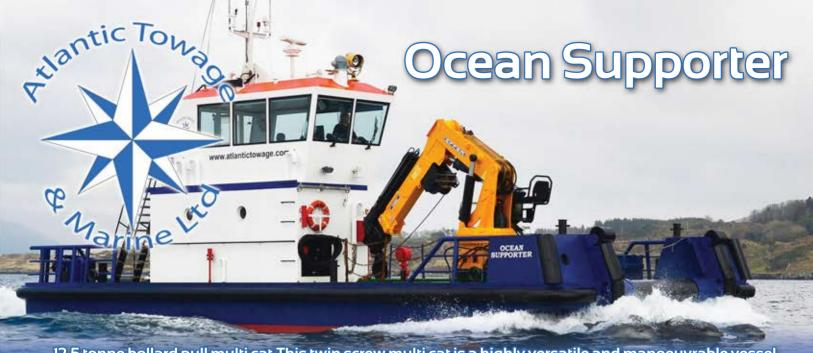
12.5 tonne bollard pull multi cat. This twin screw multi cat is a highly versatile and manoeuvrable vessel which is perfect for a variety of marine operations such as a dive support vessel, towing, anchor handling, servicing moorings and aids to navigation, assisting dredging operations, manoeuvring barges and assisting marine construction projects.
