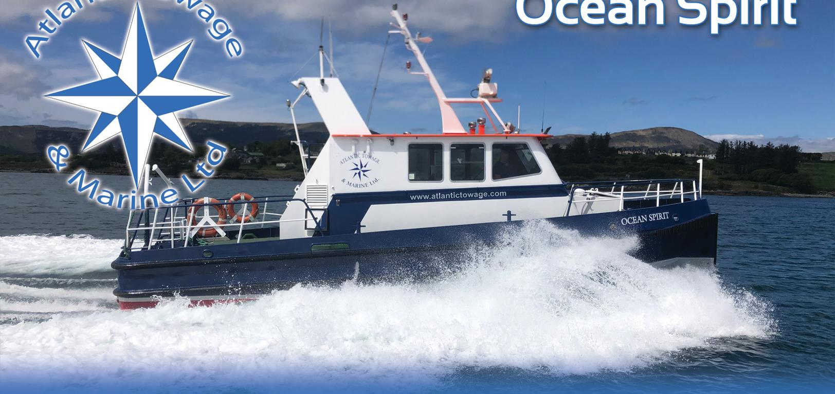
This twin screw vessel with shallow draft and large wheelhouse is ideal as a survey vessel or crew transfer vessel, also with her pusher bow this make her very useful for maneuvering barges in harbours.
